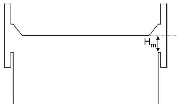
Figure 15 – Computational domain of the Configuration 3 with corrected masking height.
